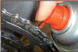
Lubricate into the chain's bearing
