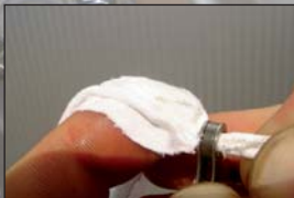
Clean inner bearing ends
